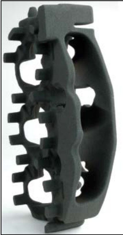
A water jacket core for an engine produced by binder jetting.
