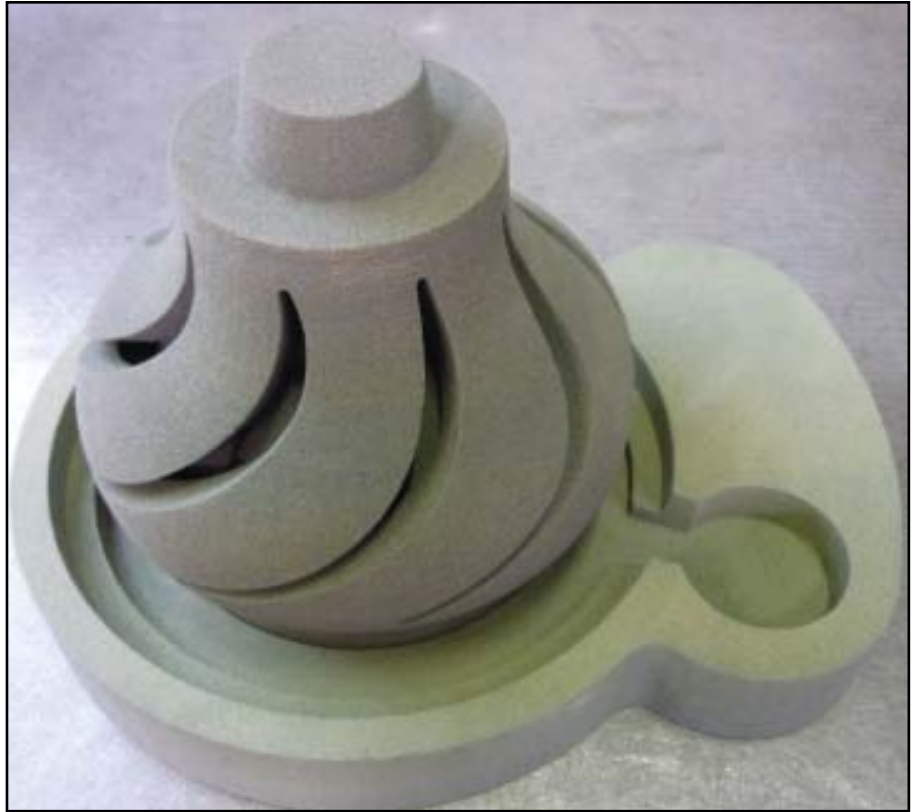
A pump impeller core produced by binder jetting.
